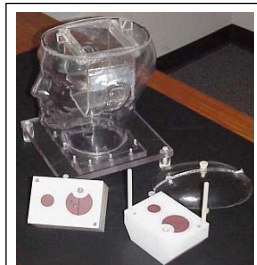
Fig. 1. RPC IMRT head and neck phantom with its insert removed and both halves of the insert separated
